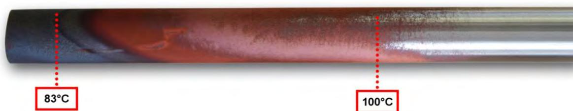
Figure 3: Deliquescence corrosion of hygroscopic salts (operation time 15 h, flue gas temperature 260°C)
