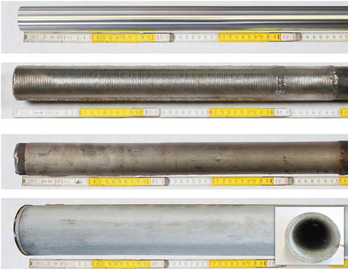
Figure 4: Material probe, application of inside thermocouples: before or after coating of the tube
